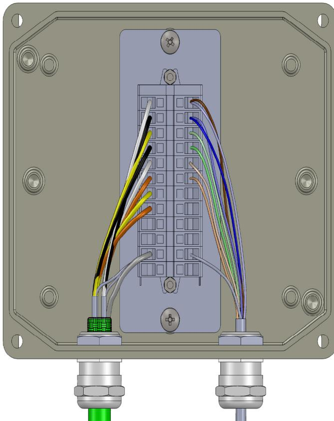
Connect the sensor cable to the Extension cable as shown. All grounds are collected together and connected to the outer ground of the Extension cable. The grounds should **not** be connected to a local ground. If there is no room for the JB12 housing, the cables can be carefully spliced together. Both cables can be cut.
