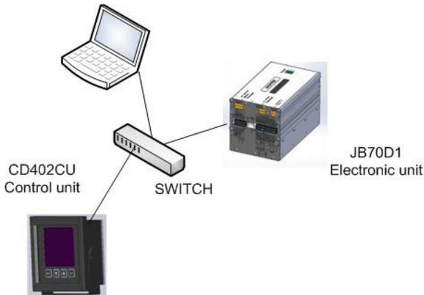
Connect the units together and use SKIPPER service software to find the relevant settings, alternatively address individual units using their IP addresses from a web browser
