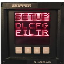
Goto setup by pressing "Menu" and "Set" at the same time. Press "down" to highlight "Filtr". Press "Set"
