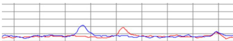
A noise top will interfere on the speed measure if larger than the speed top.
