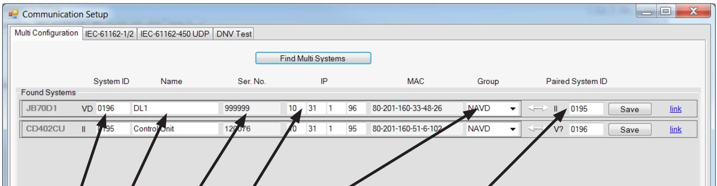
System ID of the unit that this system is to be uniquely connected to (CD402CU must have.)
