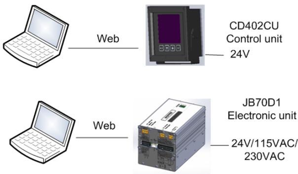
If no switch is available, connect directly to each unit and use its web page to setup. Multirepeaters can be set up directly from the screen.
